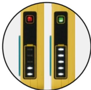
Connect the charge to the device. When the device is fully charged the green LED will be lit up
