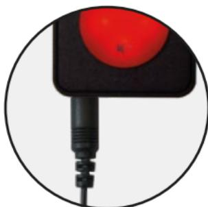
To switch on the device, connect the earphone / microphone to the receiver / transmitter
